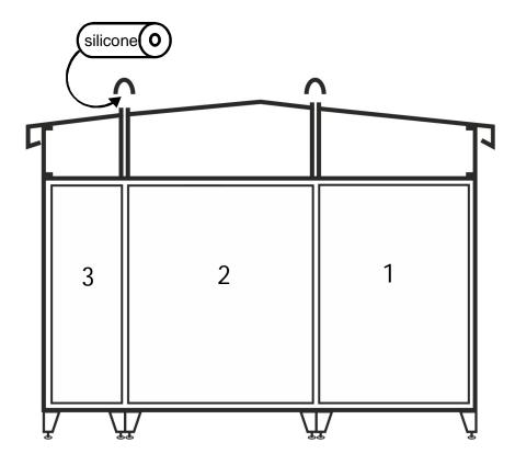
7. Seal the connections between attached U-profiles and roof plates by silicone. Seal the entire length of the connections; you will seal two connections along both ends of each U-profile.
