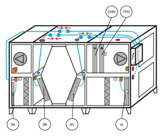
Connection of servo motors, front view
