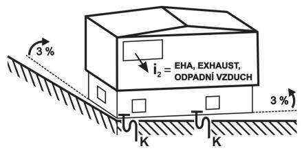
Sloping the unit towards condensate drain and towards the exhaust of stale air i2
