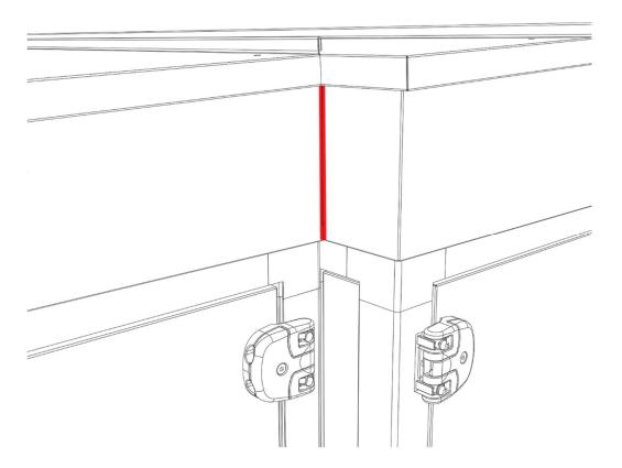
9. Seal the connection between the unit casing and the attached roof by silicone. Seal the connection all around the unit.
