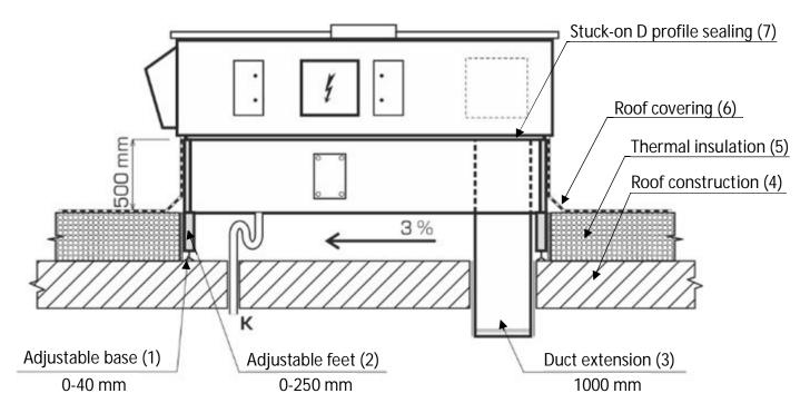
You will find the scheme of fitted unit also in the selection software of Duplexvent units. Proceed to the tab **Design**, keep the option **Base frame** selected and click on **AHU placement method**.
